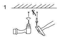
Drill holes in the ceiling and insert expansion screws
