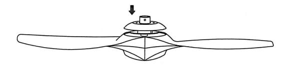
1) Fasten the six screws to secure the top cover to the connector.
